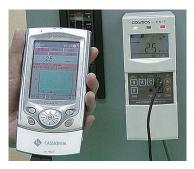
Connecting a PDA with a detector head makes it possible to acquire data stored in the head.
